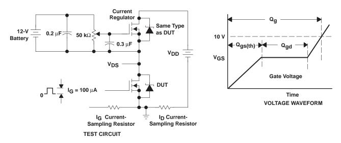
Figure 3. Gate-Charge Test Circuit and Voltage Waveform
