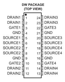
The TPIC5403 is offered in a 24-pin wide-body surface-mount (DW) package and is characterized for operation over the case temperature range of  $-40^{\circ}$ C to  $125^{\circ}$ C.
