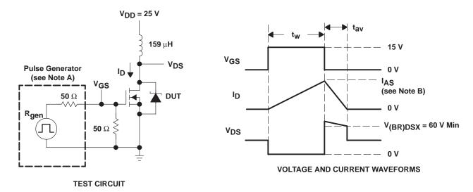
NOTES: A. The pulse generator has the following characteristics:  $t_r \le 10$  ns,  $t_f \le 10$  ns,  $z_O = 50 \Omega$ .
