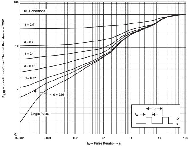
† Device mounted on 24in<sup>2</sup>, 4-layer FR4 printed-circuit board with no heatsink.
