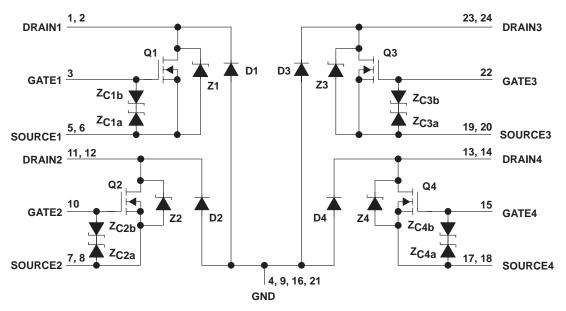
NOTE A: For correct operation, no terminal may be taken below GND.
