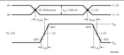
FIGURE 2. Receiver Propagation Delay and Transition Time Waveforms
