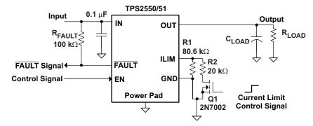
Figure 25. Two-Level Current-Limit Circuit
