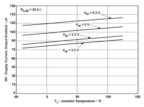
Figure 18.  $I_{\text{IN}}$  – Supply Current, Output Enabled –  $\mu\text{A}$
