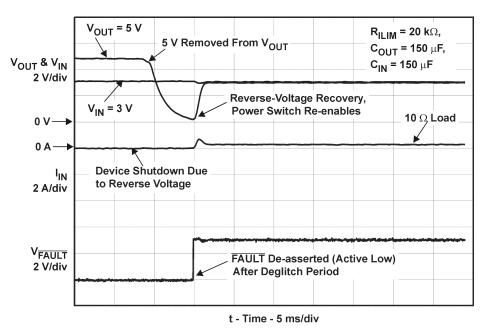
Figure 15. Reverse-Voltage Protection Recovery
