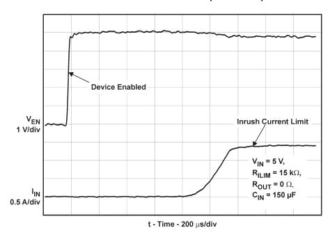
Figure 7. Device Enabled into Short-Circuit
