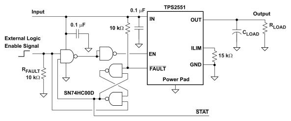
Figure 24. Overcurrent Latch-Off Using a Quad-NAND Gate
