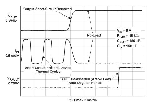
Figure 11. Short-Circuit to No-Load Recovery Response
