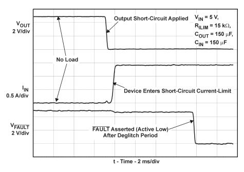
Figure 10. No-Load to Short-Circuit Transient Response
