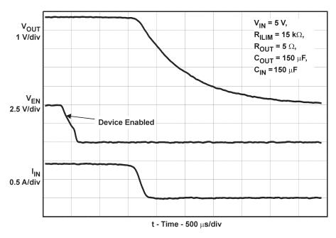
Figure 6. Turnoff Delay and Fall Time
