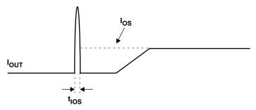
Figure 3. Response Time to Short-Circuit Waveform
