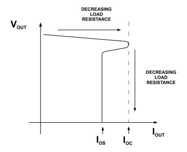
Figure 4. Output Voltage vs. Current-Limit Threshold
