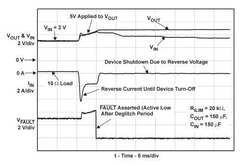
Figure 14. Reverse-Voltage Protection Response
