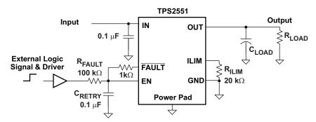
Figure 23. Auto-Retry Functionality With External EN Signal
