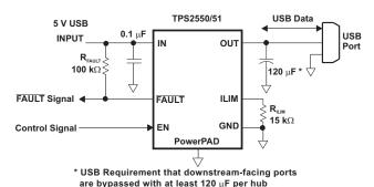
Figure 1. Typical Application as USB Power Switch
