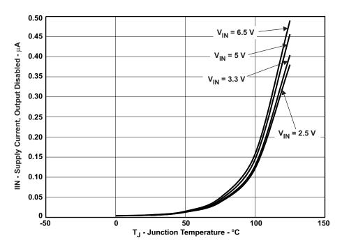
Figure 17.  $I_{\text{IN}}$  – Supply Current, Output Disabled –  $\mu$ A
