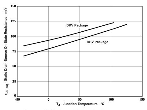
Figure 20. MOSFET  $r_{DS(on)}$  Vs. Junction Temperature
