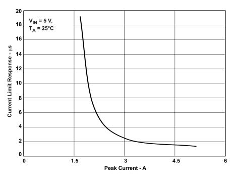
Figure 19. Current Limit Response –  $\mu$ s
