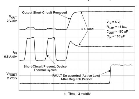
Figure 9. Short-Circuit to Full-Load Recovery Response
