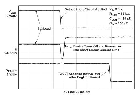
Figure 8. Full-Load to Short-Circuit Transient Response
