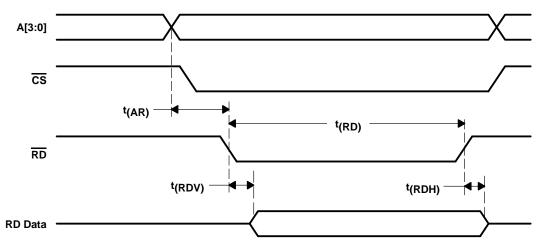
Figure 5–2. Standard ISA Read-Cycle Timing Diagram
