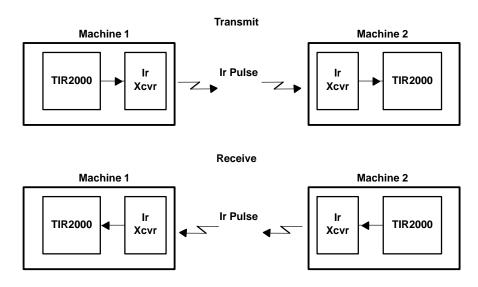
Figure 2–1. Basic Configuration for Ir Communication
