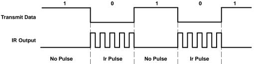
Figure 2–3. SHARP Ir Encoding
