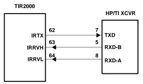
Figure 6–2. HP/TI Transceiver Connection
