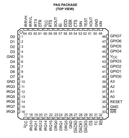
Figure 1–2. Terminal Assignments
