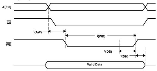
Figure 5–1. Standard ISA Write-Cycle Timing Diagram
