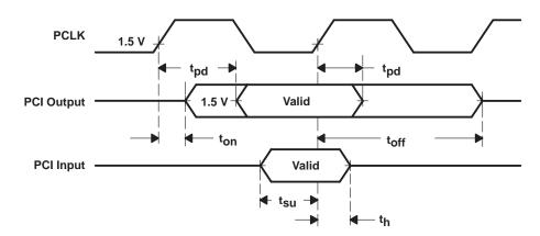
Figure 4. Shared-Signals Timing Waveforms
