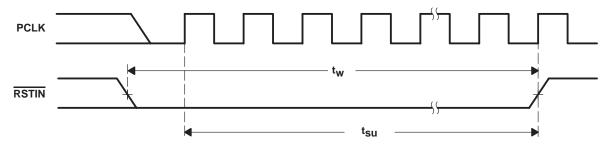
Figure 3. RSTIN Timing Waveforms
