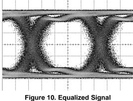
Figure 10. Equalized Signal (40 in FR4, 6.4 Gbps, PRBS31, 0x06 Setting)
