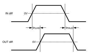
Figure 4. Propagation Delay Timing Diagram
