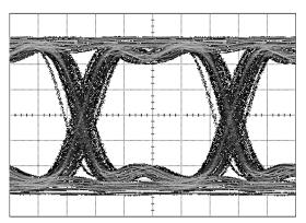
Figure 12. Equalized Signal (10m 24 AWG Twin-AX Cable, 6.4 Gbps, PRBS7, 0x06 Setting)
