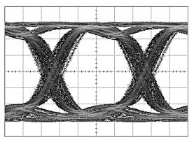
Figure 11. Equalized Signal (30 in FR4, 10 Gbps, PRBS7, 0x06 Setting)
