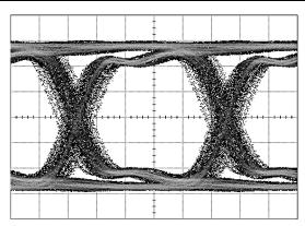
Figure 9. Equalized Signal (40 in FR4, 6.4 Gbps, PRBS7, 0x06 Setting)
