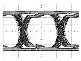
Figure 8. Equalized Signal (40 in FR4, 5 Gbps, PRBS7, 0x07 Setting)
