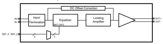
Figure 6. Simplified Block Diagram
