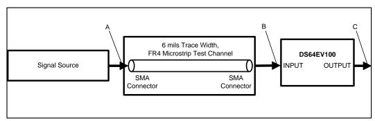
Figure 2. Test Setup Diagram
