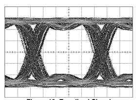
Figure 13. Equalized Signal (32 in Tyco XAUI Backplane, 6.25 Gbps, PRBS7, 0x06 Setting)
