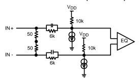
Figure 5. Simplified Receiver Input Termination Circuit
