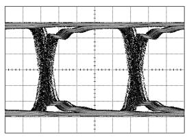
Figure 7. Equalized Signal (40 in FR4, 2.5 Gbps, PRBS7, 0x07 Setting)
