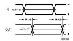
FIGURE 3. Propagation Delay Timing Diagram
