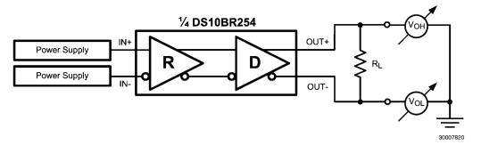
FIGURE 1. Differential Driver DC Test Circuit
