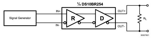
**FIGURE 2. Differential Driver AC Test Circuit**
