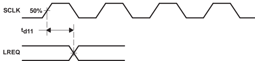
Figure 6-7. TSB12C01A Link-Request-to-Phy-Layer Waveforms
