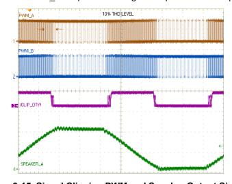
Figure 9-15. Signal Clipping PWM and Speaker Output Signals
