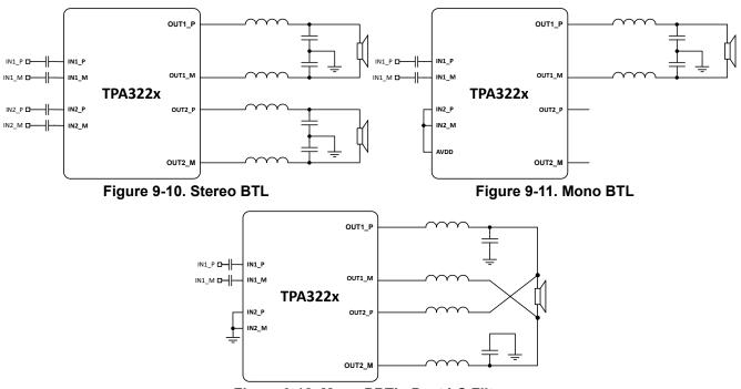
Figure 9-12. Mono PBTL, Post LC Filter
