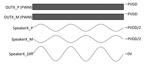
Figure 9-9. AD Mode Speaker Output Signals, Low or and High Level Output
