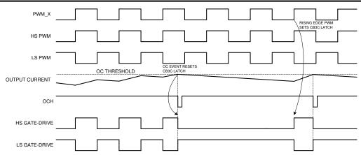
Figure 9-14. CB3C Timing Example
