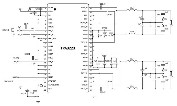
Figure 10-1. Typical Differential (2N) AD-Mode BTL Application
