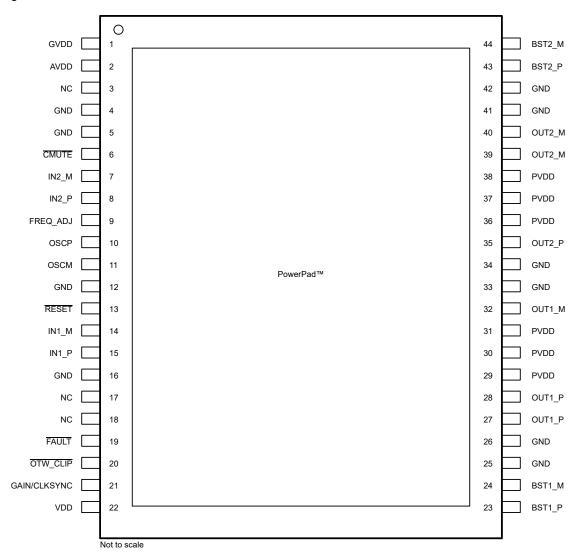
Figure 6-1. DDV Package, HTSSOP 44-Pin, Top View
