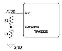
Figure 9-5. Clock Synchronization Setup
