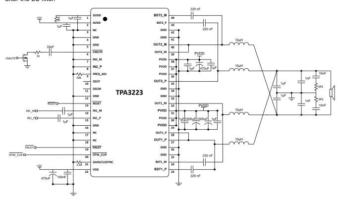
Figure 10-6. Typical Differential (2N) AD-Mode PBTL Application
