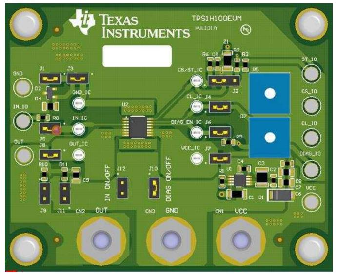
Figure 1. TPS1H100-Q1 EVM Component Placement (Top View)
