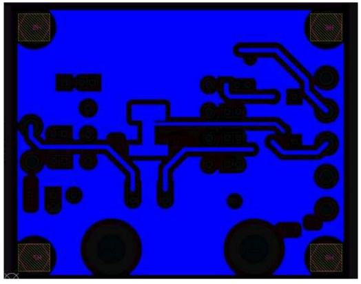
Figure 3. TPS1H100-Q1EVM Bottom Layer (Bottom View)
