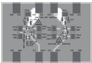
Figure 7. Bottom Layer Assembly
