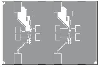
Figure 8. Top Layer Routing
