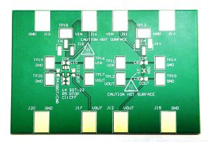
This user's guide describes the operational use of the MultiPkgLDOEVM-823 evaluation module (EVM) as a reference design for engineering demonstration and evaluation of Texas Instruments low-dropout (LDO) linear regulators, in DRB, DRV, DQN, and DBV packages. Included in this user's guide are setup and operating instructions, layout guidelines, a printed circuit board (PCB) layout, a schematic diagram, and a bill of materials (BOM).
