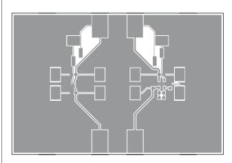
Figure 9. Bottom Layer Routing
