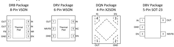
Figure 1. Supported Packages and Pinouts
