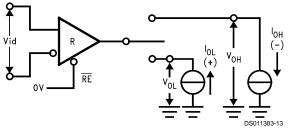
FIGURE 12. Receiver  $V_{\rm OH}$  and  $V_{\rm OL}$
