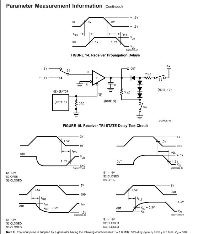
**Note 9:**  $C_L$  includes probe and stray capacitance.
