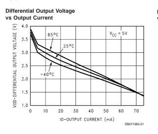
Differential Output Voltage vs Output Current
