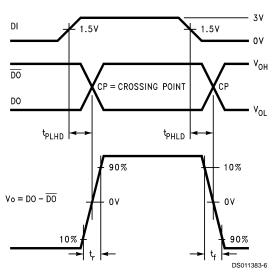
FIGURE 5. Driver Differential Propagation Delays and Transition Times
