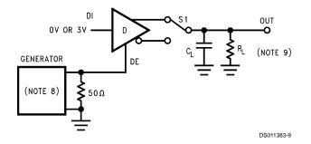
S1 to DO for DI = 3V S1 to  $\overline{DO}$  for DI = 0V
