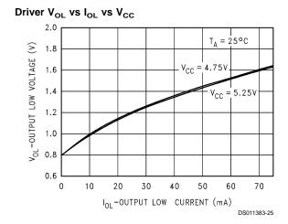
Driver VoL vs IoL vs Temperature
