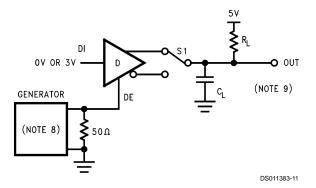
S1 to DO for DI = 0V S1 to  $\overline{DO}$  for DI = 3V
