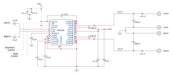
Figure 27. Schematic for Single-Ended (SE) Configuration
