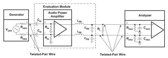
Figure 31. Differential Input, BTL Output Measurement Circuit
