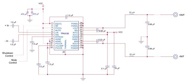
Figure 28. Schematic for Bridge-Tied (BTL) Configuration
