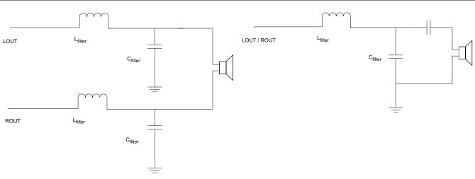
Figure 25. BTL Filter Configuration
