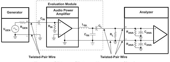
Figure 30. SE Input—SE Output Measurement Circuit
