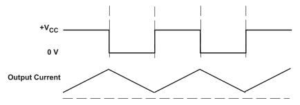
Figure 23. Class-D Modulation for TPA3120D2 SE Configuration
