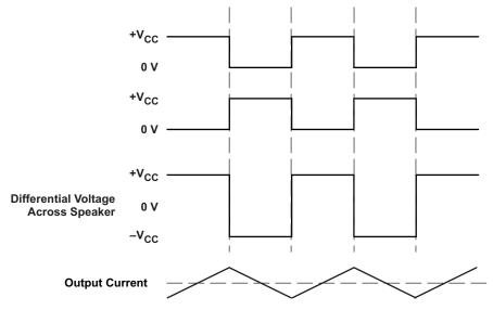
Figure 24. Class-D Modulation for TPA3120D2 BTL Configuration
