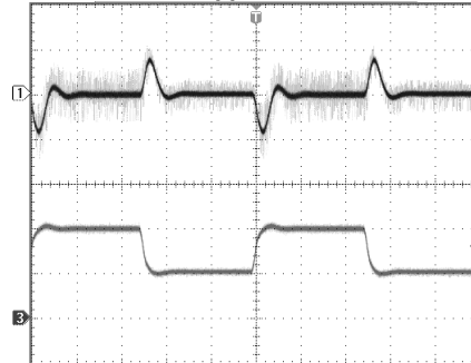
V_{OUT} = 8.5V , V_{IN} = 3.3V , C_{OUT} = 20\mu F 1) V_{OUT} , 200mV/div, AC 3) I_{LOAD} , 200mA/div, DC T = 200\mu s/div
