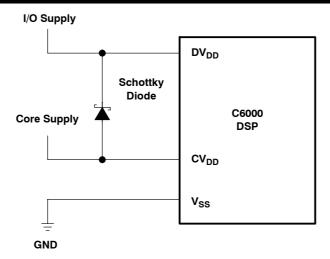
Figure 11. Schottky Diode Diagram
