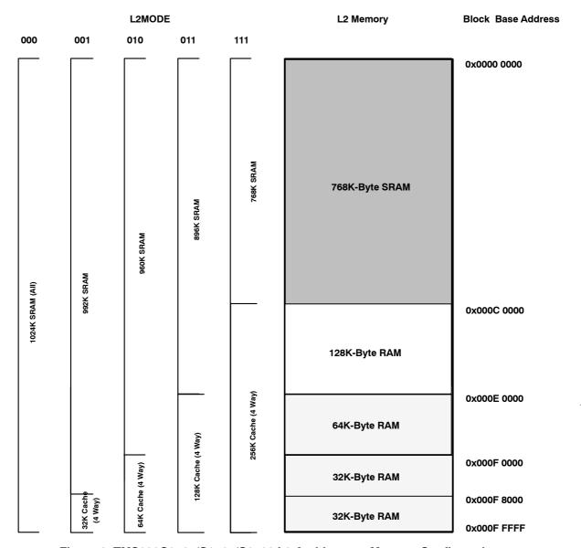
Figure 2. TMS320C6414/C6415/C6416 L2 Architecture Memory Configuration
