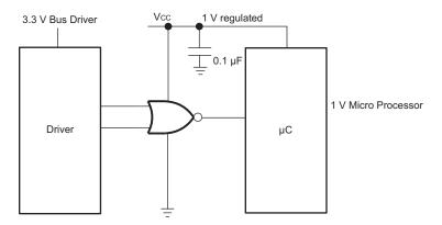
Figure 5. Typical Application Schematic
