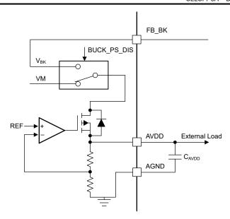
Figure 7-7. AVDD Linear Regulator Block Diagram
