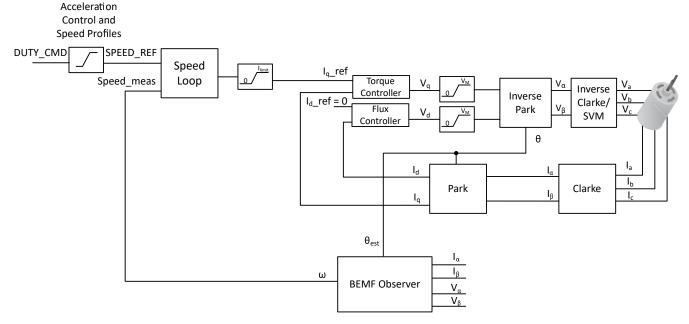
Figure 7-33. Closed Loop FOC Control
