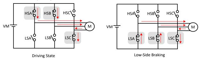
Figure 7-47. Low-Side Braking
