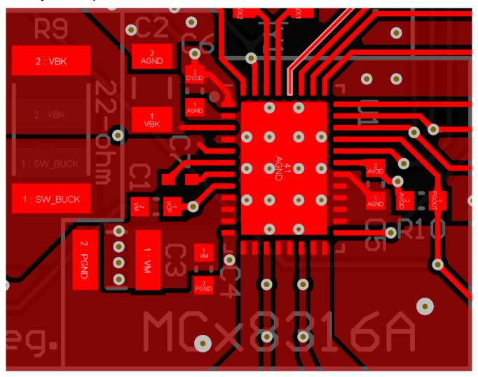
Figure 10-1. Recommended Layout Example
