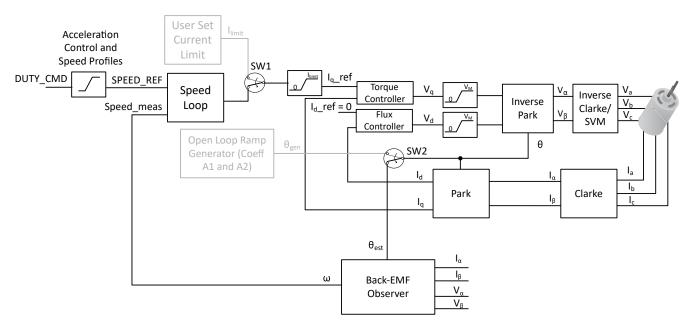
Figure 7-32. Open to Closed Loop Transition Control Block Diagram
