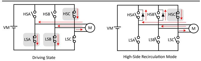
Figure 7-46. High-Side Recirculation
