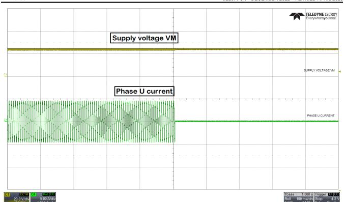
Figure 8-9. Motor stop - recirculation mode
