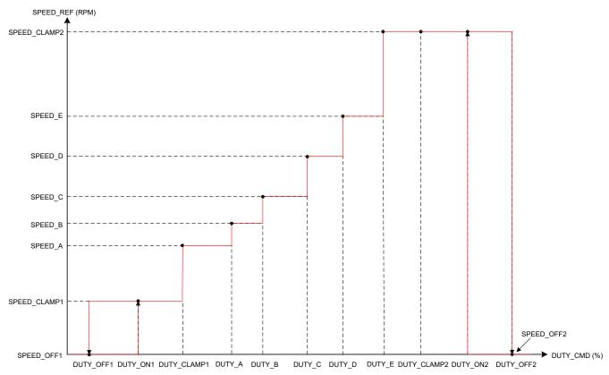
Figure 7-20. Staircase Speed Profile
