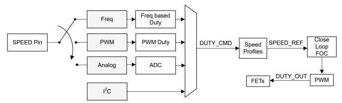
Figure 7-13. Multiplexing the Speed Command
