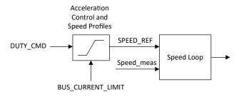
Figure 7-51. DC Bus Current Limit Functional Block Diagram
