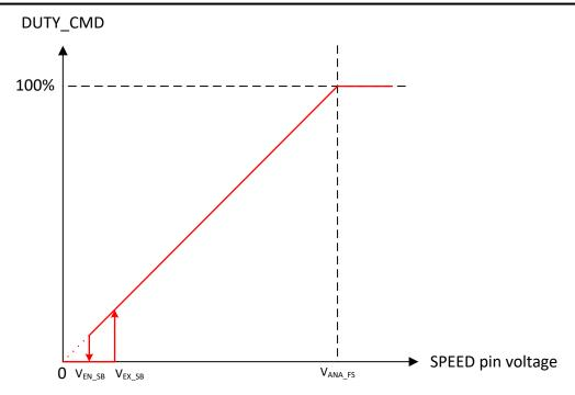
Figure 7-14. Analog Mode Speed Control
