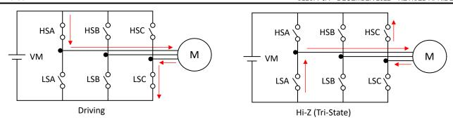
Figure 7-28. IPD Release Mode - Tristate (1b)
