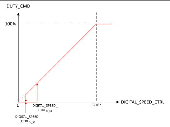
Figure 7-16. I2C Mode Speed Control
