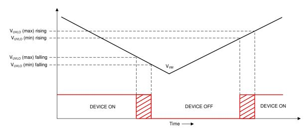
Figure 7-52. VM Supply Undervoltage Lockout
