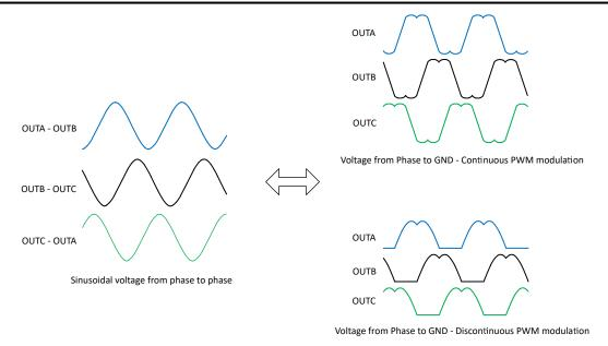
Figure 7-43. Continuous and Discontinuous PWM Modulation Phase Voltages
