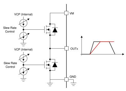
Figure 7-9. Slew Rate Circuit Implementation
