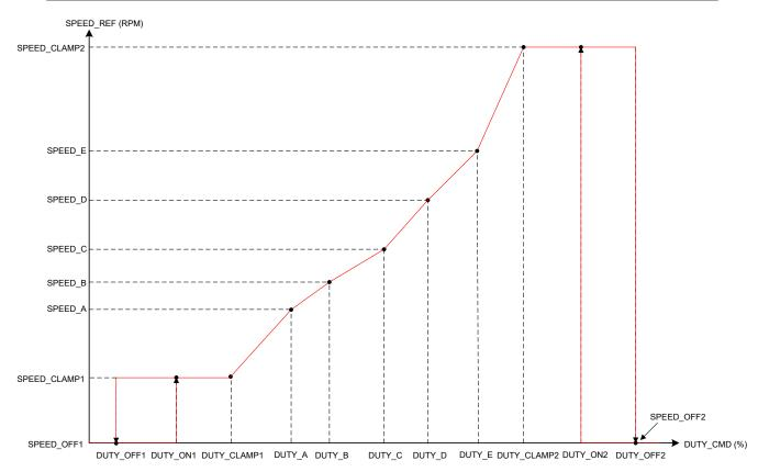
Figure 7-19. Linear Speed Profile
