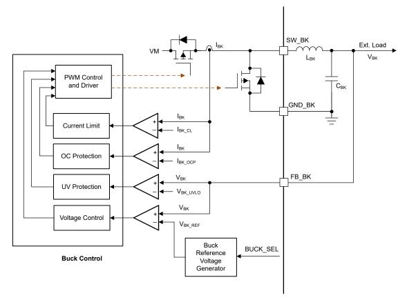
Figure 7-6. Buck Operation and Control Loops
