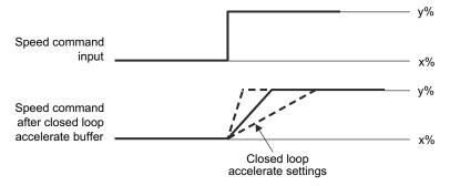
Figure 7-34. Closed loop accelerate
