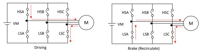
Figure 7-27. IPD Release Mode - Brake (0b)
