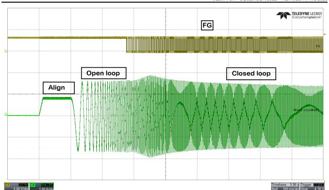
Figure 8-3. Motor Startup - FG and Phase current
