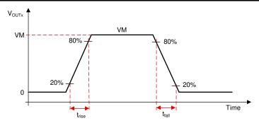
Figure 7-10. Slew Rate Timings
