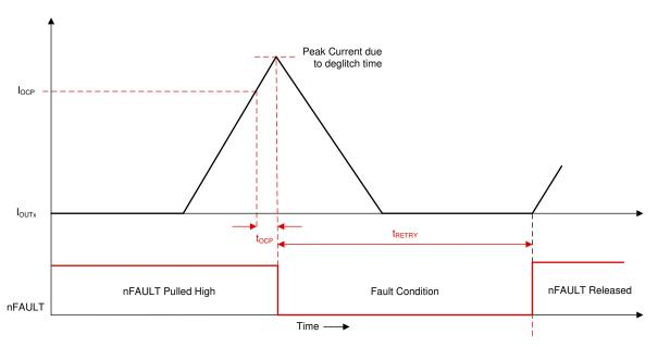
Figure 7-55. Overcurrent Protection - Automatic Retry Mode
