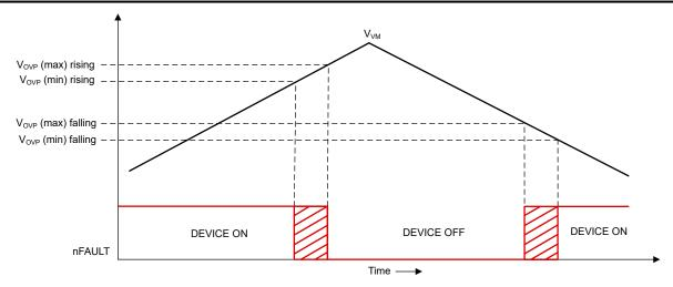
Figure 7-53. Over Voltage Protection
