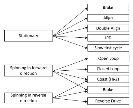
Figure 7-22. Starting the motor under different initial conditions
