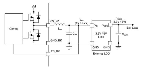
Figure 7-4. Buck Regulator with External LDO
