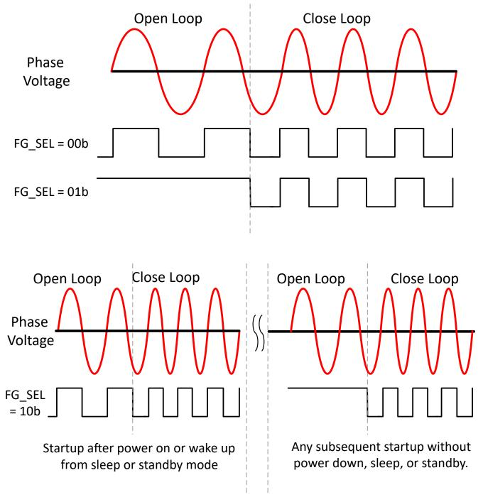
Figure 7-50. FG Behavior During Open Loop
