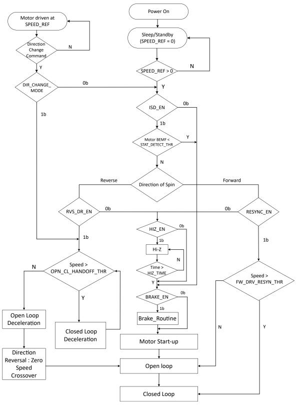
Figure 7-23. Motor Start Sequence
