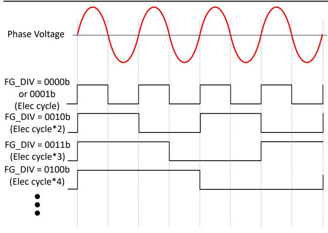
Figure 7-49. FG Frequency Divider
