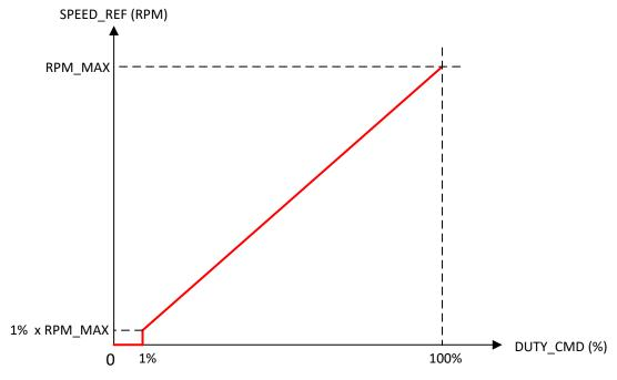
Figure 7-18. Speed reference (SPEED\_PROFILE\_CONFIG = 00b)
