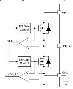
Figure 7-11. Cross Conduction Protection
