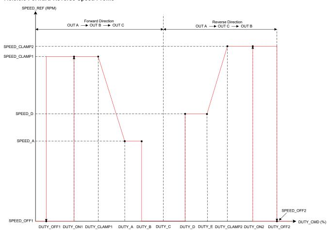
Figure 7-21. Forward-Reverse Speed Profile
