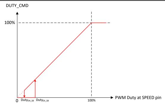
Figure 7-15. PWM Mode Speed Control
