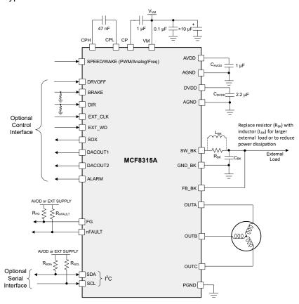
Figure 8-1. Example Application Schematic
