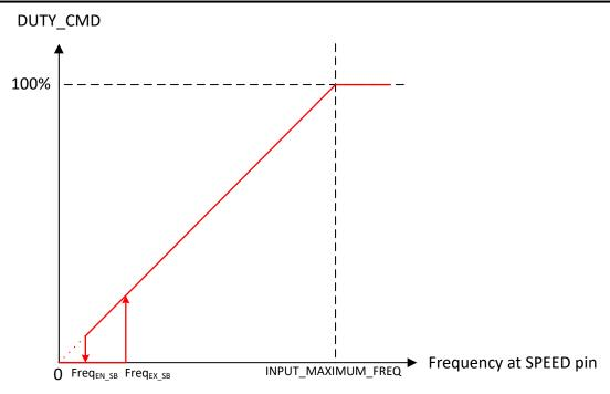
Figure 7-17. Frequency Mode Speed Control
