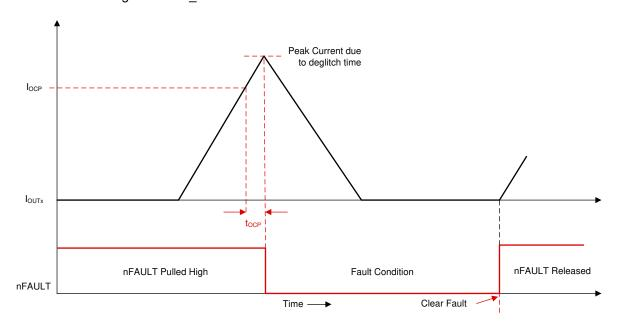
Figure 7-54. Overcurrent Protection - Latched Shutdown Mode
