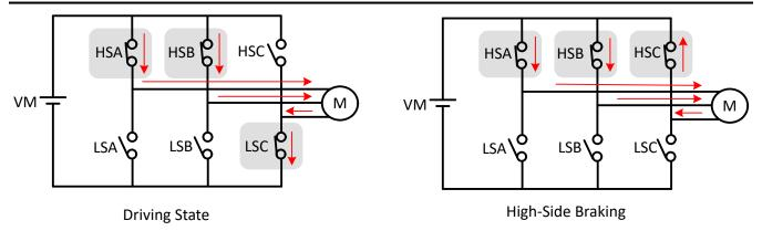
Figure 7-48. High-Side Braking
