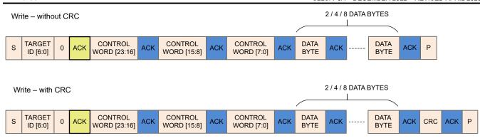
Figure 7-57. I<sup>2</sup>C Write Transaction Sequence
