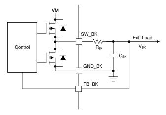
Figure 7-3. Buck (Resistor Mode)
