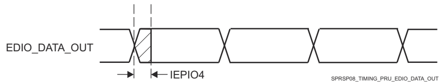
Figure 7-106. PRU_ICSSG PRU IEP Digital IOs Timing
