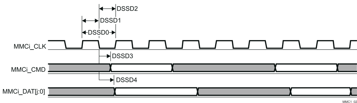
Figure 7-73. eMMC/SD/SDIO in - Default Speed - Transmitter Mode
