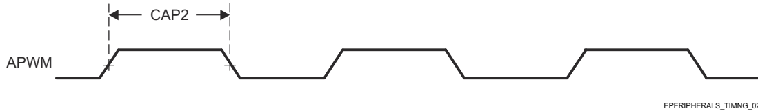
Figure 7-42. eCAP Switching Characteristics
