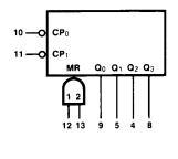
V<sub>CC</sub> = Pin 14 GND = Pin 7 NC = Pins 1, 2, 3, 6
