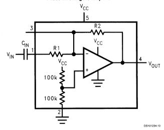
$V_{OUT} = 0.5V_{CC} - V_{IN} (R_2/R_1)$
