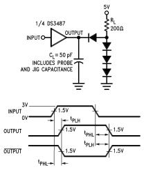
Input pulse: f = MHz, 50%;  $t_r = t_f \le 15$  ns.
