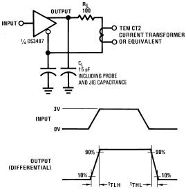
Input pulse: f = MHz, 50%;  $t_r = t_f \le 15$  ns.
