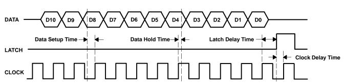
NOTE: Data is clocked in on the positive edge of the clock. The positive edge of the latch signal should occur before the next positive edge of the clock. For definition of D0 to D10, see the control logic table.
