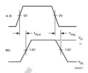
FIGURE 9. Receiver Propagation Delay
