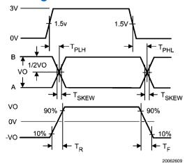
FIGURE 7. Driver Propagation Delay, Rise / Fall Time
