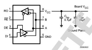
FIGURE 11. Placement of by-pass Capacitors, C<sub>bp</sub>
