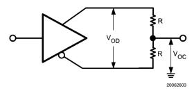
FIGURE 1. Test Circuit for  $\rm V_{OD}$  and  $\rm V_{OC}$
