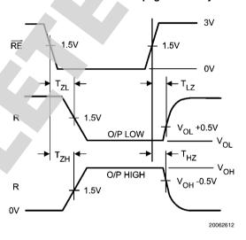
FIGURE 10. Receiver Enable / Disable Time
