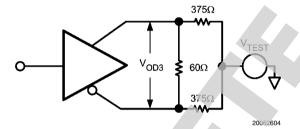
FIGURE 2. Test Circuit for V<sub>OD3</sub>
