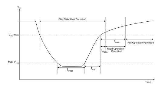
Figure 24. Power-Up Timing
