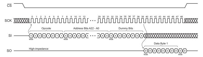
Figure 40. Continuous Array Read (Opcode 0Bh)
