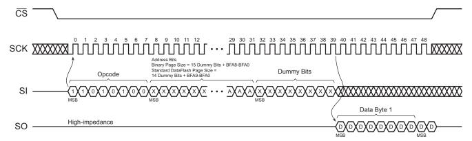
Figure 43. Buffer Read (Opcode D4h or D6h)
