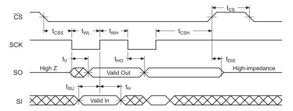
Figure 29. Waveform 2 = SPI Mode 3 Compatible
