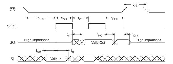
Figure 28. Waveform 1 = SPI Mode 0 Compatible
