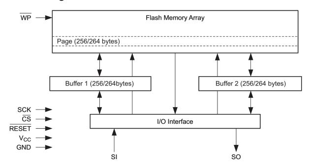
Figure 2. AT45DB641E Block Diagram
