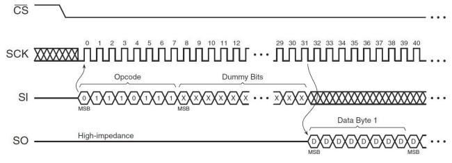
Figure 47. Read Security Register (Opcode 77h)
