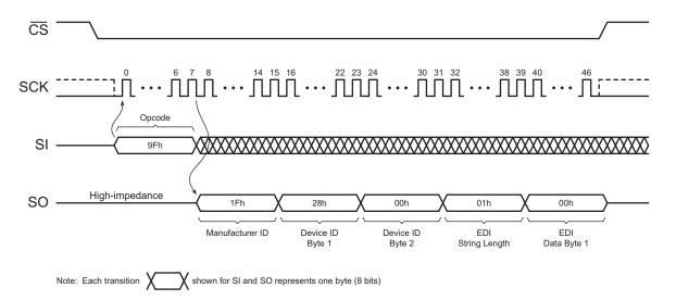
Figure 22. Read Manufacturer and Device ID
