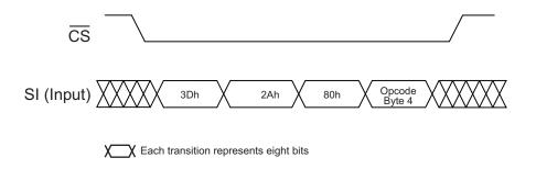
Figure 21. Buffer and Page Size configuration
