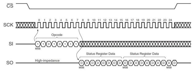
Figure 48. Status Register Read (Opcode D7h)
