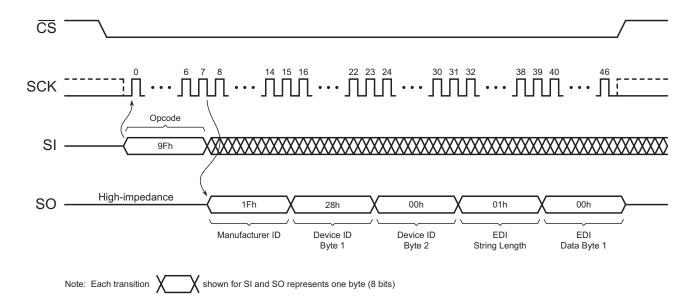
Figure 49. Manufacturer and Device Read (Opcode 9Fh)
