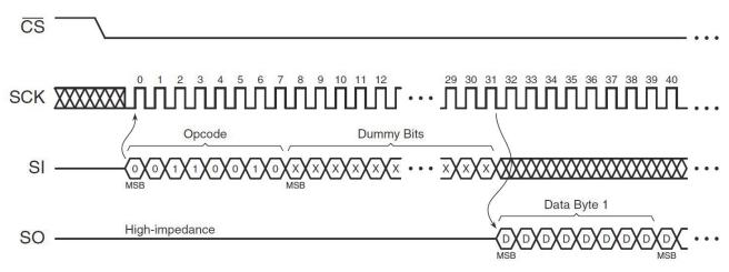
Figure 45. Read Sector Protection Register (Opcode 32h)
