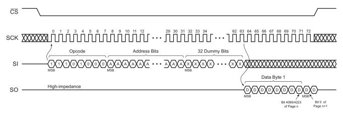
Figure 39. Continuous Array Read (Legacy Opcode E8h)
