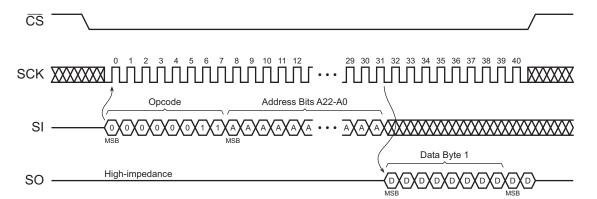
Figure 41. Continuous Array Read (Opcode 01h or 03h)
