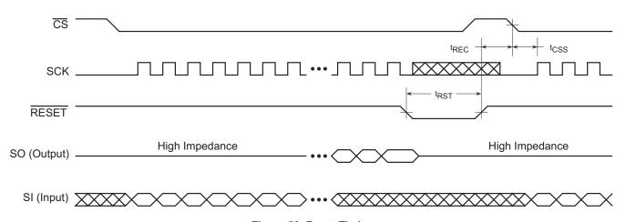
Figure 50. Reset Timing
