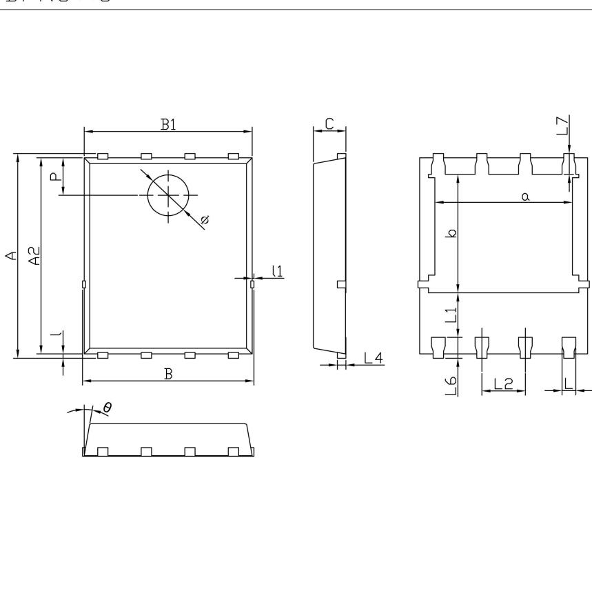
The technical drawing illustrates the physical dimensions of the PDFN5×6 package. It includes three views: a top view showing the overall footprint, a side view showing the height and lead spacing, and a cross-sectional view showing internal features like the thickness and lead profile. Dimensions are labeled as follows:
