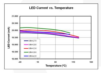
Figure 6. LED Current Variation vs. Temperature
