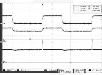
Figure 12. Line Transient Response in 1.5x Mode,  $V_{IN}$ =2.7 V – 3.3 V,  $I_{LED}$ =20 mA
