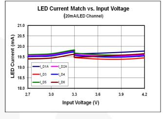
Figure 5. LED Current Match for all 6 LED Channels at I<sub>LED</sub>=20 mA
