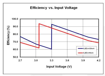
Figure 4. Efficiency with LED Current of 8 mA and
