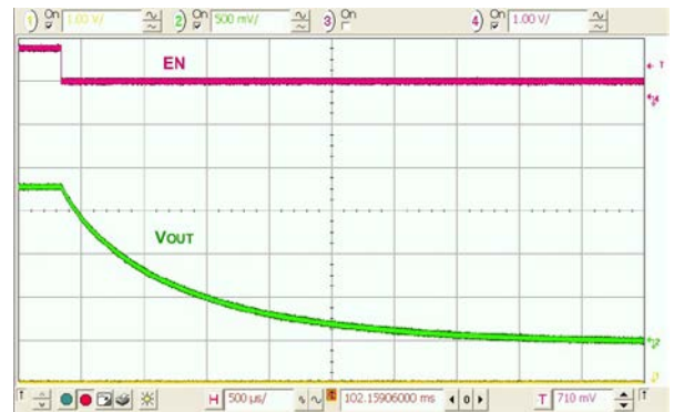
Figure 27. Shutdown, No Load, Output Discharge Enabled
