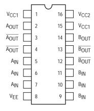
Pin assignment is for Dual–in–Line Package.
