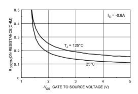
Figure 3. On-Resistance Variation with Temperature.
