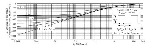
Figure 11. Transient Thermal Response Curve.
