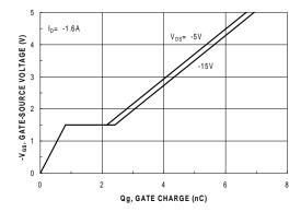
Figure 7. Gate Charge Characteristics.
