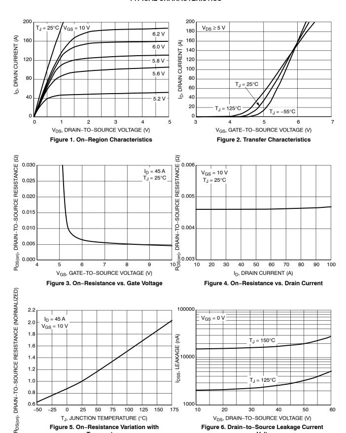
Figure 6. Drain-to-Source Leakage Current
