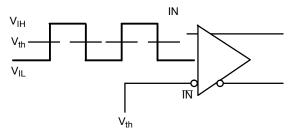
Figure 5. Differential Input Driven Single-Ended
