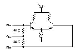
Figure 4. Input Structure
