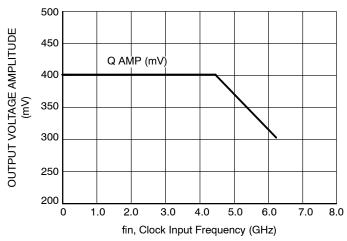
Figure 3. CLOCK Output Voltage Amplitude (V<sub>OUTPP</sub>) vs. Input Frequency (f<sub>in</sub>) at Ambient Temperature (Typ)
