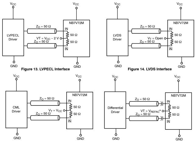
Figure 15. Standard 50  $\Omega$  Load CML Interface
