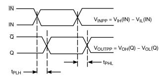
Figure 10. AC Reference Measurement
