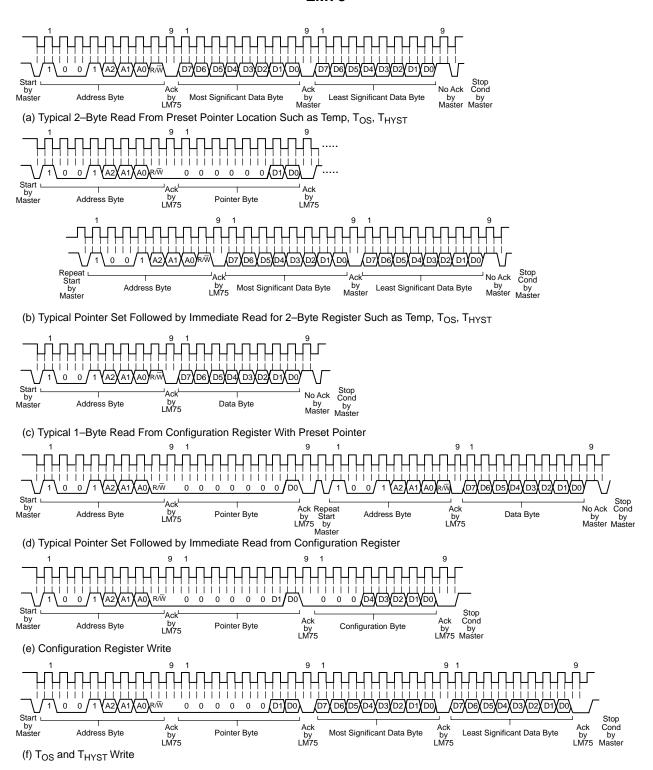
Figure 2. Serial Port Operation
