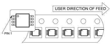
Standard Reel Component Orientation for R2 Suffix Device (Mark Right Side Up)
