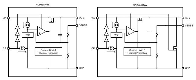
Figure 2. Simplified Schematic Block Diagram
