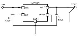
Figure 39. Typical Application Schematic
