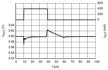
Figure 29. Load Transients, 3.6 V Version, Load Step 1 mA to 400 mA
