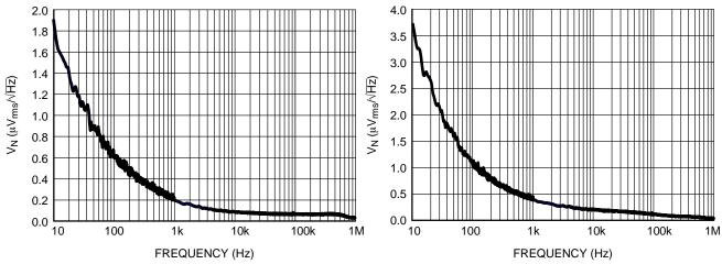
Figure 21. Output Noise vs. Frequency, 0.7 V Version
