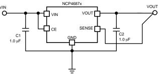
Figure 1. Typical Application Schematic
