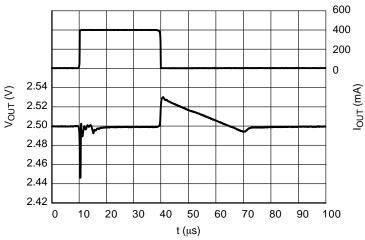
Figure 28. Load Transients, 2.5 V Version, Load Step 1 mA to 400 mA
