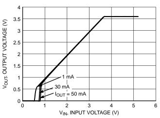
Figure 7. Output Voltage vs. Input Voltage 2.5 V Version
