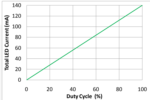
Figure 11. Total LED Current vs. PWM Duty Cycle, I_{LED} = 5 \times 28\text{ mA}
