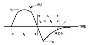
Figure 14. Diode Reverse Recovery Waveform
