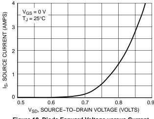
Figure 10. Diode Forward Voltage versus Current
