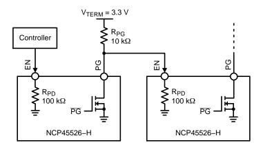
Figure 5. NCP45526 Simplified Application Diagram – Power Sequencing with PG Output
