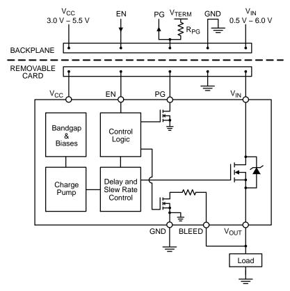
Figure 4. NCP45526 Typical Application Diagram - Hot Swap
