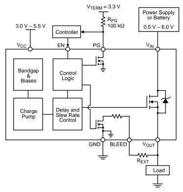
Figure 3. NCP45526 Typical Application Diagram - Load Switch
