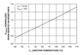
Figure 3. On-Resistance Variation with Temperature.
