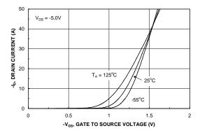
Figure 5. Transfer Characteristics.
