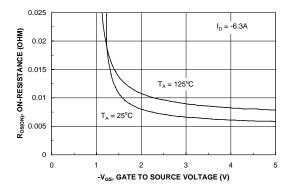
Figure 4. On-Resistance Variation with Gate-to-Source Voltage.
