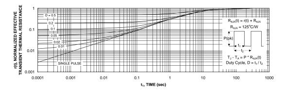
Figure 11. Transient Thermal Response Curve.
