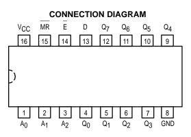
MC54/74F259 8-BIT ADDRESSABLE LATCH FAST<sup>™</sup> SCHOTTKY TTL **J SUFFIX** CERAMIC CASE 620-09 **N SUFFIX** PLASTIC CASE 648-08 D SUFFIX SOIC CASE 751B-03 **ORDERING INFORMATION** MC54FXXXJ Ceramic MC74FXXXN Plastic MC74FXXXD SOIC LOGIC SYMBOL 14 15 MR D 13 -1 A<sub>0</sub> 2 A<sub>1</sub> A2 3  $Q_4$  $Q_6$ Q7 Q<sub>0</sub>  $Q_2$ Q1 Qa Q5
