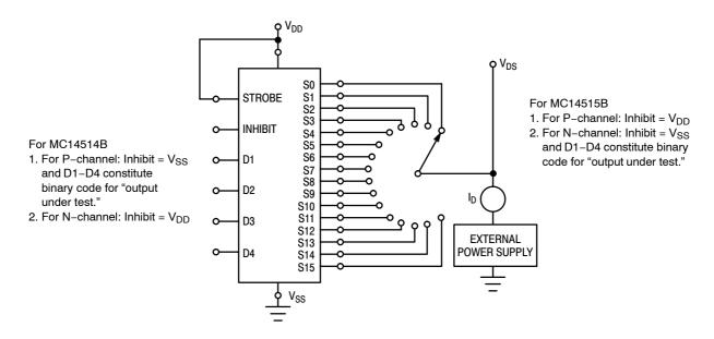
Figure 1. Drain Characteristics Test Circuit
