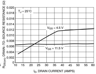
Figure 3. On-Resistance vs. Gate-to-Source Voltage
