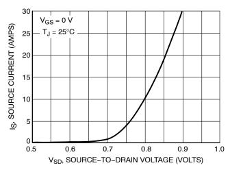
Figure 10. Diode Forward Voltage vs. Current
