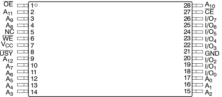
TSOP Package (8 mm x 13.4 mm) (H13)
