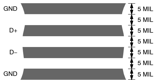
Figure 23. Typical Arrangement of Signal Tracks
