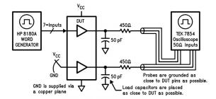
Figure 2. Simultaneous Switching Test Circuit
