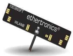
BT Tunable FPC 2.4 GHz Embedded Antenna with cable
