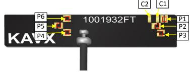
\*This antenna has unique features enabling limited range RF tuning by leaving P1 - P6 and C1 - C2 connected by "solder bridge" or disconnected with a "cut" to the trace. Refer to detailed tuning options below.
