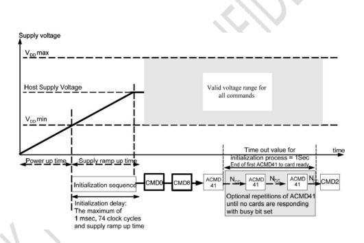
'Power up time' is defined as voltage rising time from 0 volt to VDD min.
