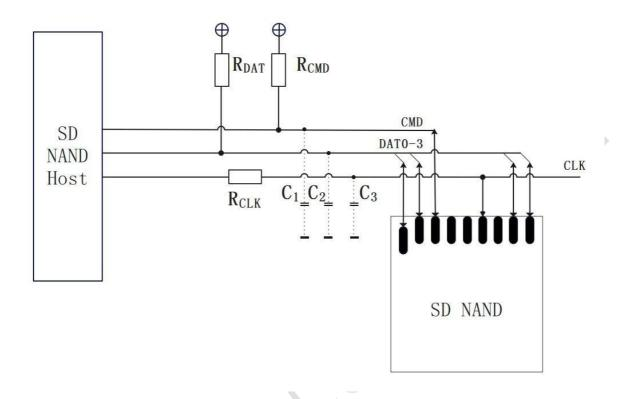
RDAT and RCMD (10K~100 k $\Omega$ ) are pull-up resistors protecting the CMD and the DAT lines against bus floating when Nano SD NAND is in a high-impedance mode.
