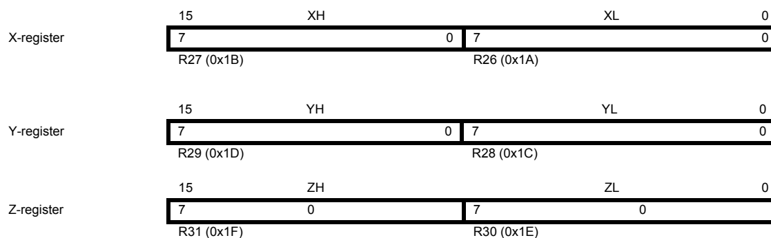
Figure 7-3. The X-, Y- and Z-registers.
