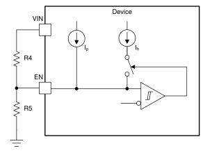
Figure 7-1. Adjustable VIN Undervoltage Lockout
