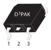
1—Gate 2—Drain 3—Source Backside—Drain
