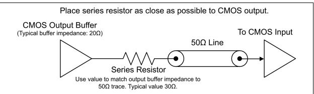
FIGURE 3-1: Typical CMOS Termination.
